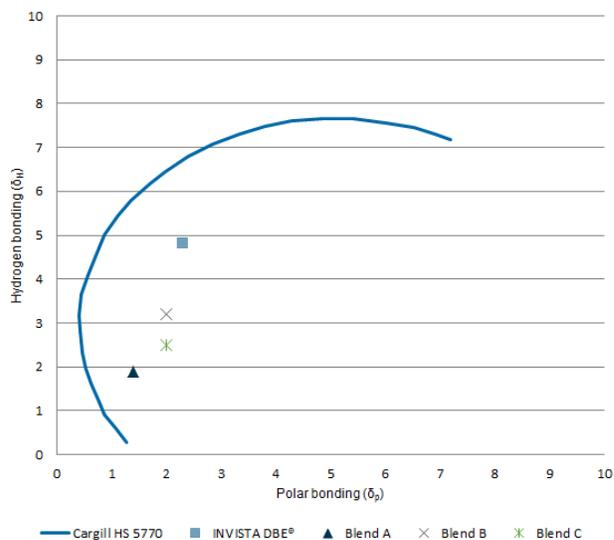
Another aid in formulating with DBE® esters uses the solubility parameter concept to choose the best combination and concentration of solvents for blending with DBE® esters. The region, or envelope, of solubility of the resin or resin mixture is determined by examining resin solubility in a series of solvents having known solubility characteristics. A plot of resulting data shows the
